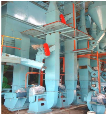
Figure 1: 4-stage winnowing column
