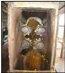
EFB Roller Crusher (30HP) To loosen and remove the fruitlets from hard and unstripped bunches ↓
