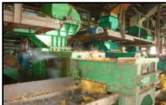
EFB Shredder & EFB Press (75HP) -to shred before press machine -to extract the press liquor from bunch - moisture content in EFB after press – 50 – 55% - oil content EFB after press– 0.2 – 0.3 to FFB
