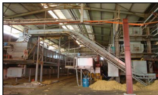
Hammer Mill (50HP) - to break down fibre into single fibre strands →
